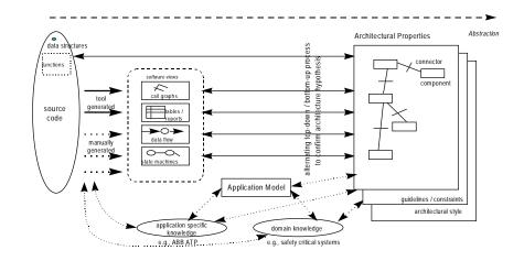
Figure 1: Framework for Architecture Recovery
